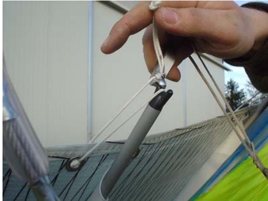
Use included lever tool to properly slip batten ties over batten tips.
