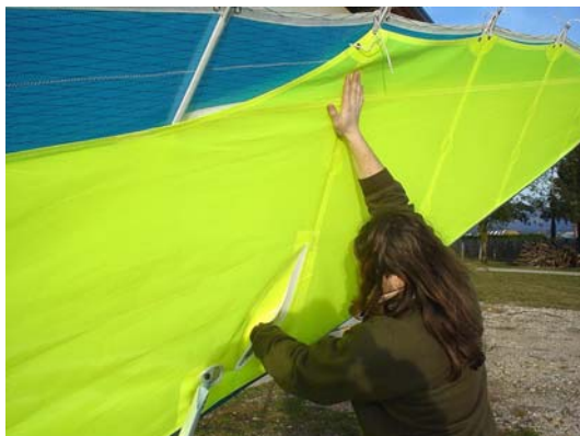
To help slip the slotted end over the keeper, push the trailing part of the sprog tube as shown with one hand. The other hand will position the slotted end over and under the keeper nut. Now release pressure on the sprog end and the slotted end should lock into place under the nut.
