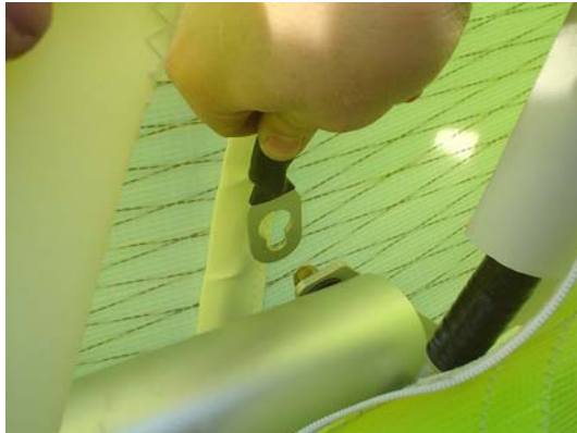
Grasp bungeed wire and slip slotted end over the nut on the keeper.
