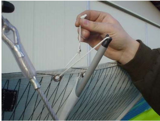
Begin attachment of batten ties
