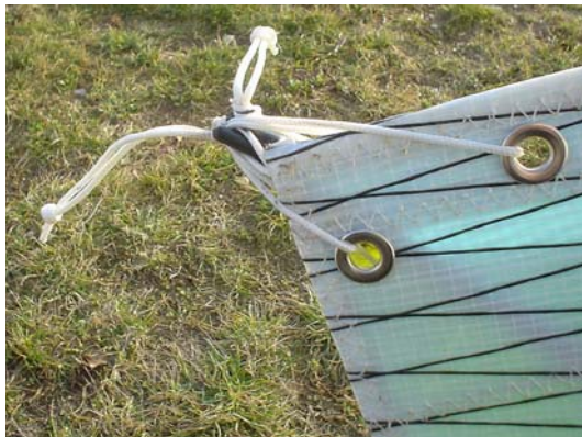
Detailed photo of properly installed tip batten.
