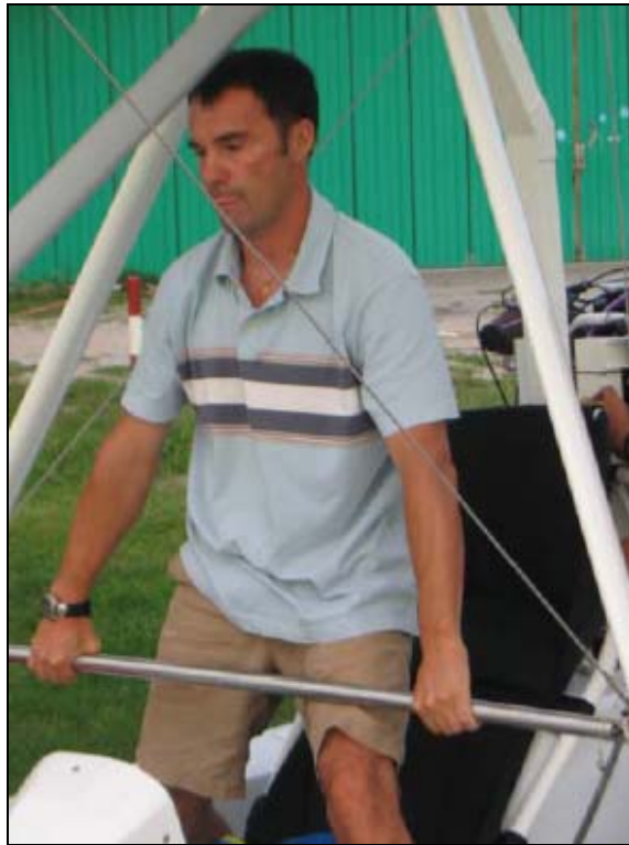
Step 12. Control bar must be raised as helper prepares to re-install bolt at forward compression strut bracket.
