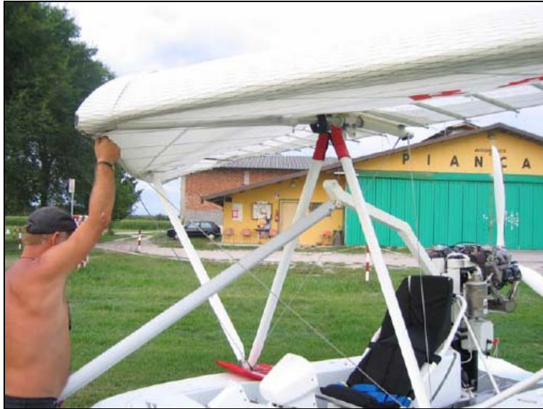
Step 7. Helper must raise nose to put hang block in position to mate with mast.
