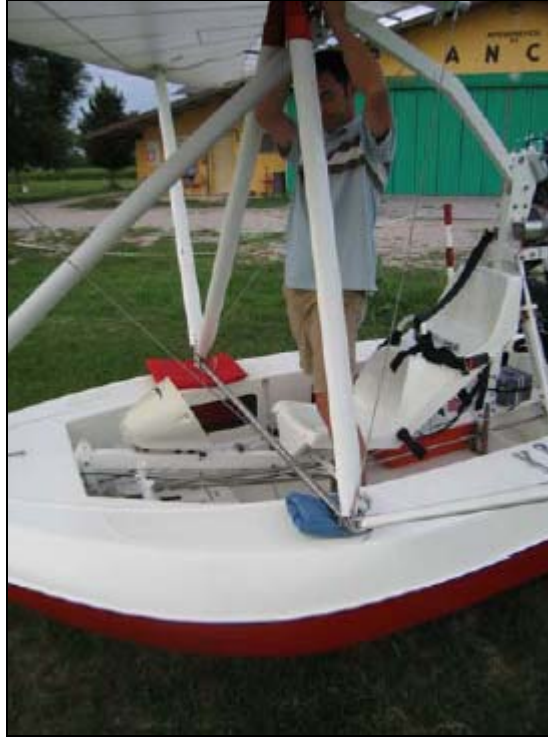
Step 9. Holes for hang block should be lined up with upper mast hole.
