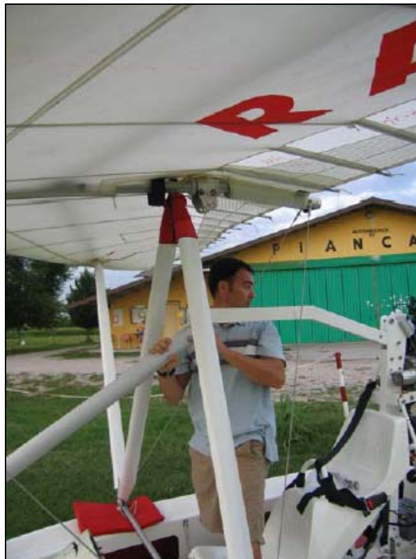
Step 8. Mast must now be raised to hang block.
