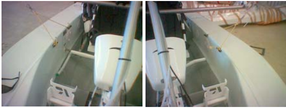
TYPE 1 HULL NO INBOARD CUTOUTS
