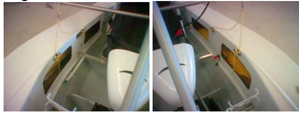
TYPE 2 HULL WITH INBOARD CUTOUTS
